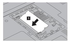
8. Push the SO-DIMM down until it snaps into place.
